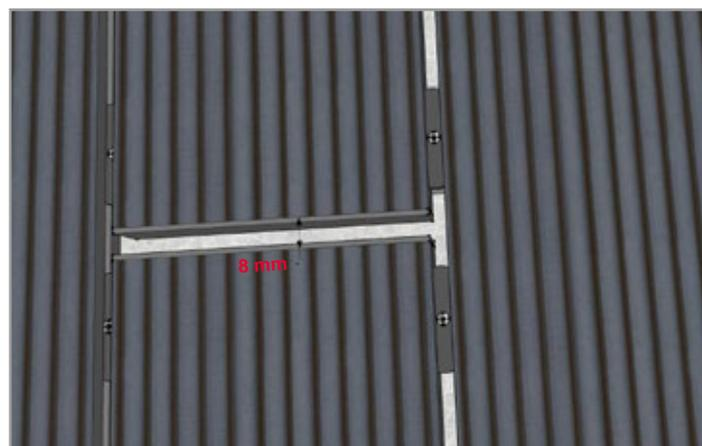
mm, while the joist structure to which the slats are to be screwed must have a maximum centre distance of 350mm. Lift the frame at the intersection points of the aluminium joists using the 8 mm rubber shims, which SKEMA has in the price list. SKEMA technical office is available to evaluate the best solution with the designer, taking into consideration the construction site situation.
